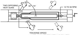
1/2" TO 1"/MINUTE FOR METALLIC ROLLERS 1" TO 1-1/2" /MINUTE FOR NON-METALLIC ROLLERS
